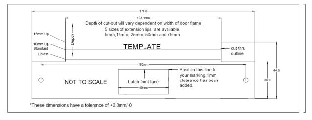
If the frame is not prefabricated, use the enclosed stick-on template to prepare strike cut-out in frame. Install strike as described in diagram.
