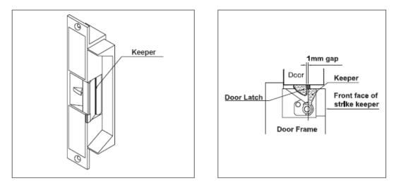
As drawn in the diagrams, there should be a 1mm gap between the door latch and the front-face of the strike keeper, preventing the door from creating back pressure on the strike keeper when the door is closed.
